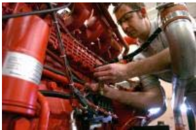
Cameron Alberts, an engine lab technician for Woodward Governor Co. in Loveland, tests a fuel-metering valve the company makes. The valve is used on natural-gas bus engines. (Lyn Alweis, The Denver Post )
